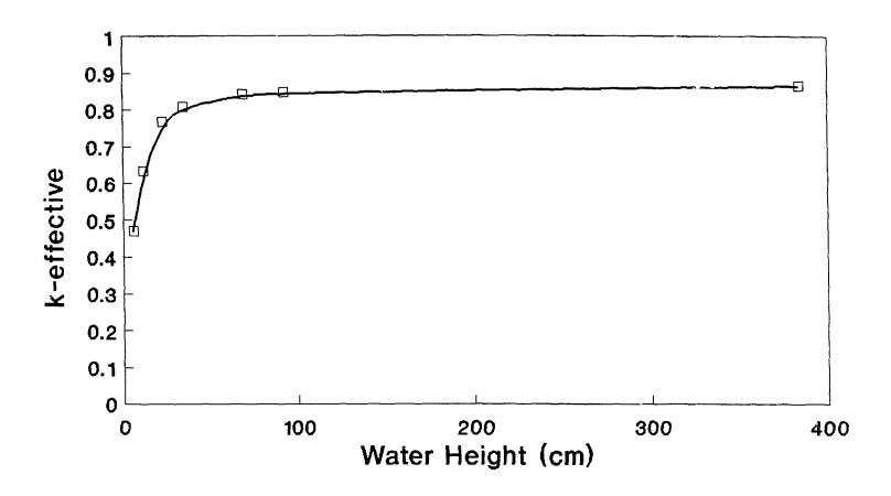
Fig. 1. keff results from cask reflooding event.
