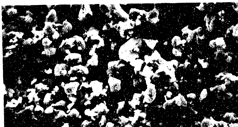
Fig. 2.3. Scanning electron micrograph of metal diboride powders (1000 \times ). (a) TiB_2 , (b) HfB_2 , (c) ZrB_2 .
