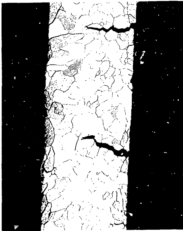
Fig. 13. Cross section containing the cracks seen in Fig. 12. 50X.
