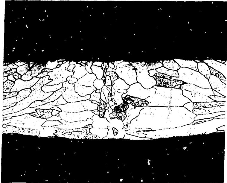
Fig. 12. Microstructure of the single-pass weld section taken from SRP-127, 50X.
