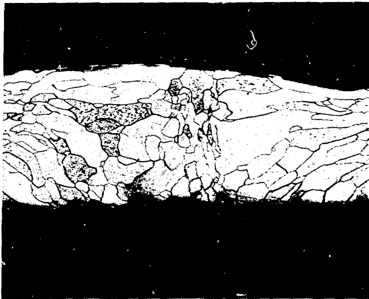
Fig. 21. The single-pass weld section taken from SRP-317 had a typical microstructure, 50X.
