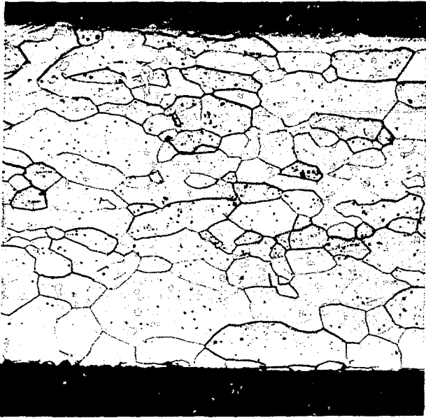
Fig. 31. Microstructure of a specimen removed from the vent cup of capsule SRP-251, 100X.
