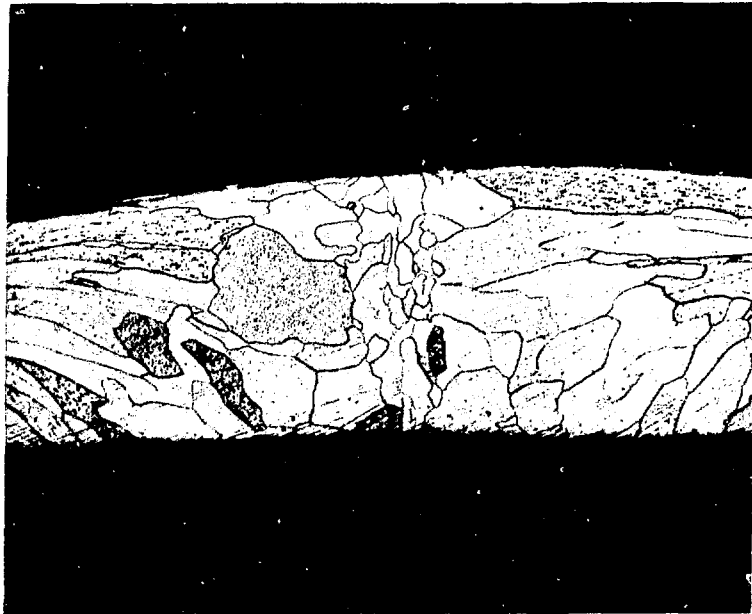
Fig. 18. The single-pass weld specimen removed from capsule SRP-251 had a typical microstructure, 50X.
