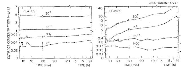
Figure 3. Dissolution kinetics of several ions from particles deposited on inert plates and on leaves. In practice, all leaves are extracted for 3 minutes to maximize removal of external deposits and minimize removal of internal material. Inert plates are extracted for 30 minutes, although 5 minutes would be sufficient to remove essentially all soluble ions.
