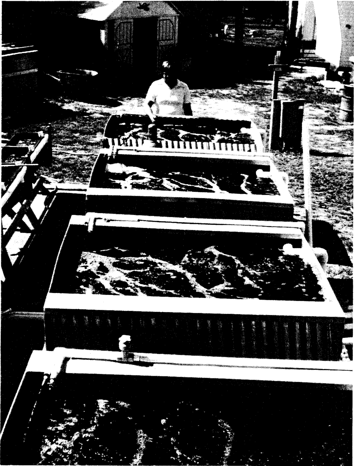
Figure 6 2400-liter aluminum culture tanks used for nutrient recycling experiments.
