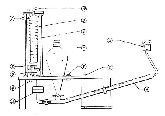
Fig. 3.1. Vibrating orifice system for the production of controlled-size, monodispersed aerosol particles supplied to the microcombustor; code: 1. dilution N<sub>2</sub>; 2. dispersion N<sub>2</sub>; 3. piezoelectric ceramic vibrator; 4. from signal generator; 5. electrical heater; 6. main body; 7. liquid solution storage; 8. dispersion flow regulator. 9. signal amplifier switch; 10. pressure regulator; 11. volumetric flow-meter; 12. filter (0.5  $\mu$ m); 13. aerosol to pressurized combustor.
