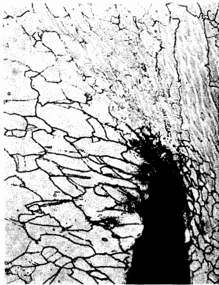
FIGURE 10. Weld Area of the Impacted Hastelloy C-4 Capsule
