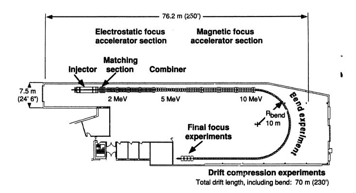
Figure 2. Diagram of the ILSE accelerator and principal experiments that will examine the induction linac approach to a driver.
