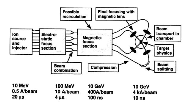
Figure 1. Schematic of a conceptual accelerator/driver that delivers  $4\times10^{14}$  W of heavy ions for 10 ns. The total length of the facility is expected to be 5–10 km.
