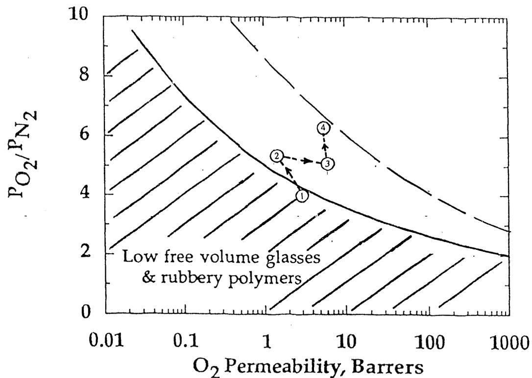
Figure 2: Permeability-Selectivity Tradeoff Relationship for the oxygen-nitrogen system with a "trajectory" formed by consideration of the structures "1"-8" in Table 2. The significance of the solid and dashed boundaries are discussed in the text.
