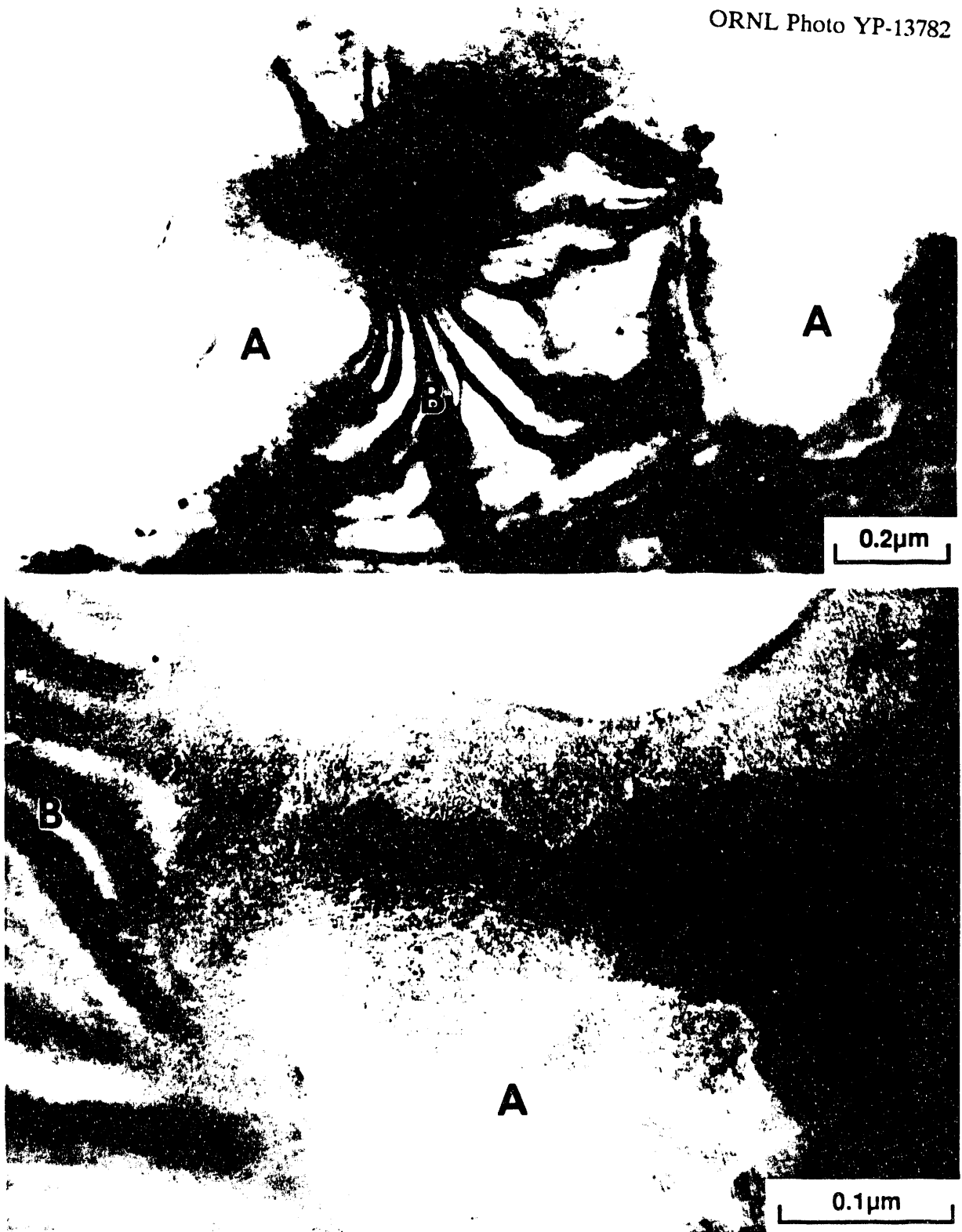
Fig. 8.12. Transmission electron micrographs showing regions where only corrosion material (primarily goethite) remain (A) and where corrosion material coats single-crystalline pyrite (B).
