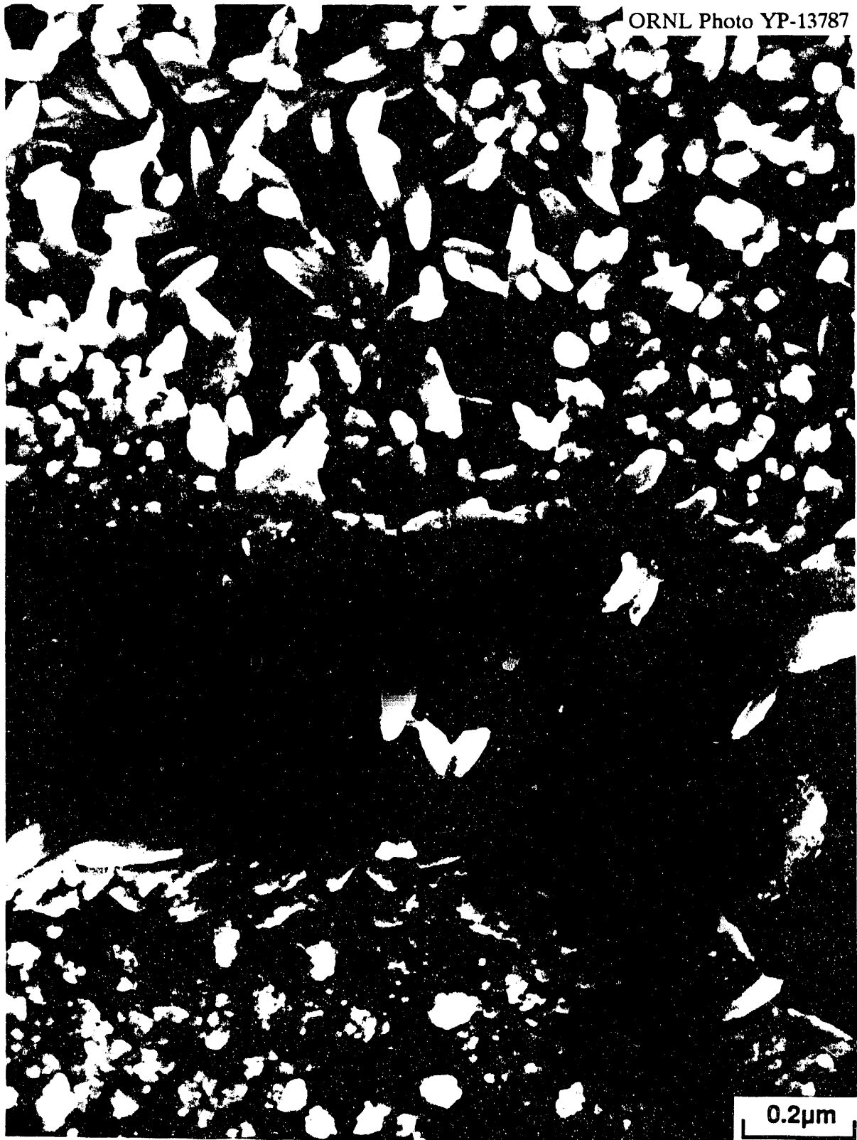
Fig. 8.11. High magnification scanning electron micrograph showing particles and crystallites that comprise the central portions of many of the corrosion pads.
