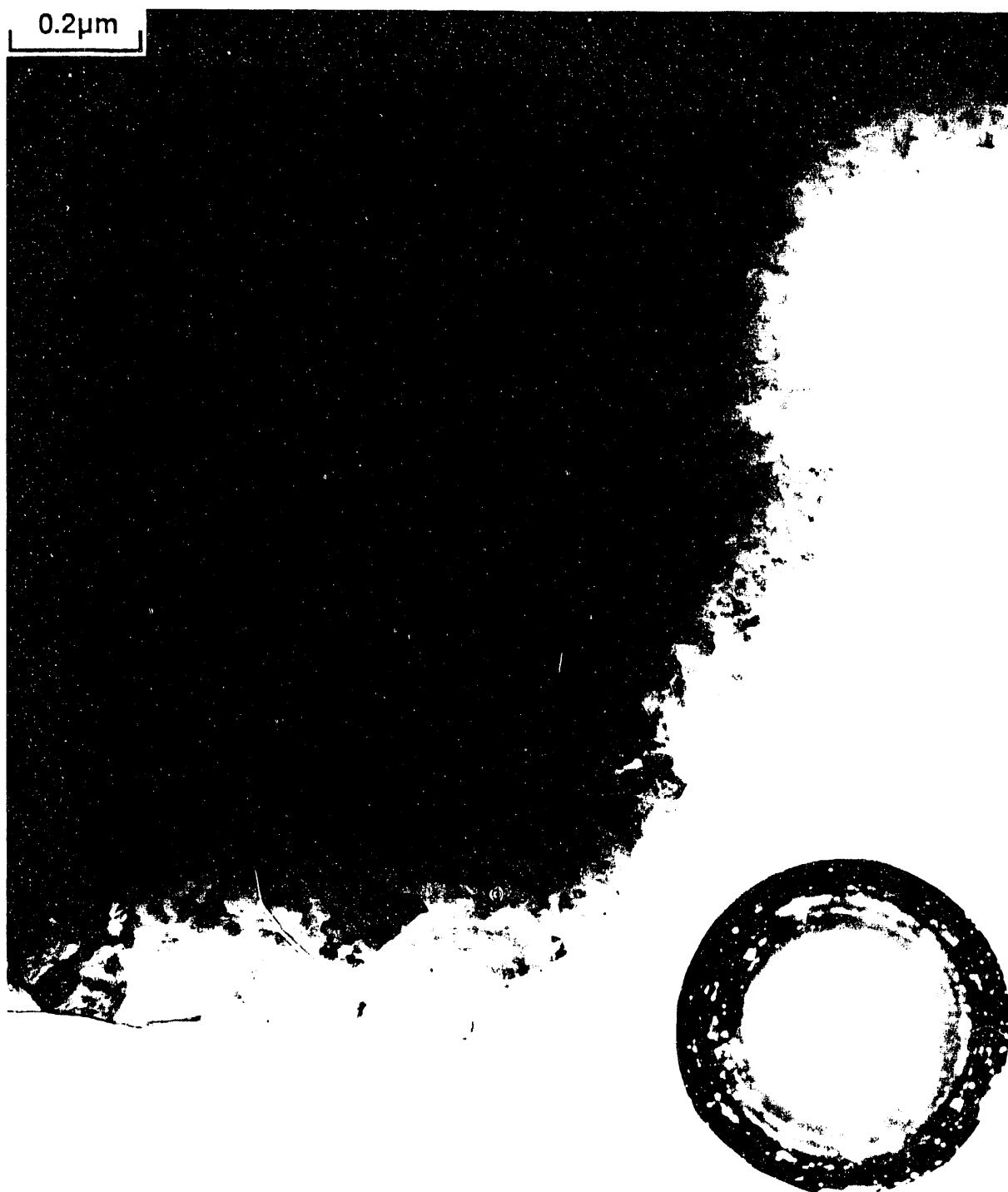
Fig. 8.8. TEM image of a bulk cube-shaped crystal sectioned through the center of the crystal, looking normal to the cube face (a \langle 100 \rangle direction). The internal structure of this crystal is polycrystalline (confirmed by the ring nature of the inset electron diffraction pattern) with a grain size of 10 to 50 nm.
