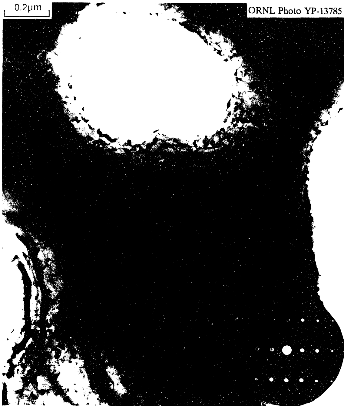
Fig. 8.9. TEM image of a bulk cube-shaped crystal sectioned through a near-surface layer, looking normal to the cube face as in Fig. 8.8. The structure at the surface of the crystal is single crystalline, as indicated by the inset electron diffraction.
