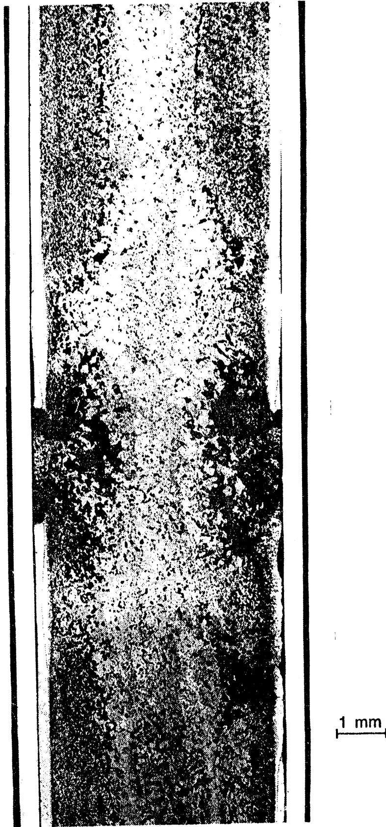
Figure 4. Longitudinal section of a Zr-sheathed U-20.5Pu-3Zr element near X/L = 0.50 .
