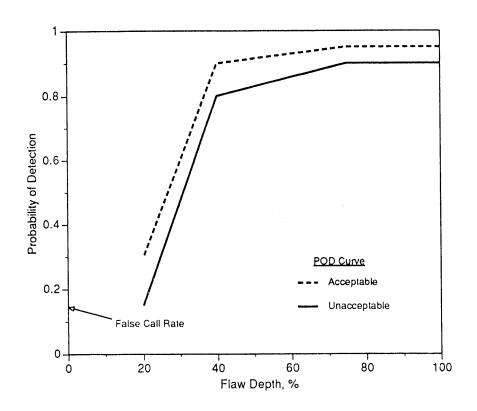
Fig. 3 Base Case Threshold POD Curves
