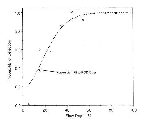
Fig. 1 Example POD Curve
