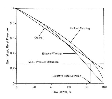
Fig. 2 Plot of Burst Mode Failure Pressure Equations Ver. us Flaw Destit for 0.775 in. CD x 0.050 in.
