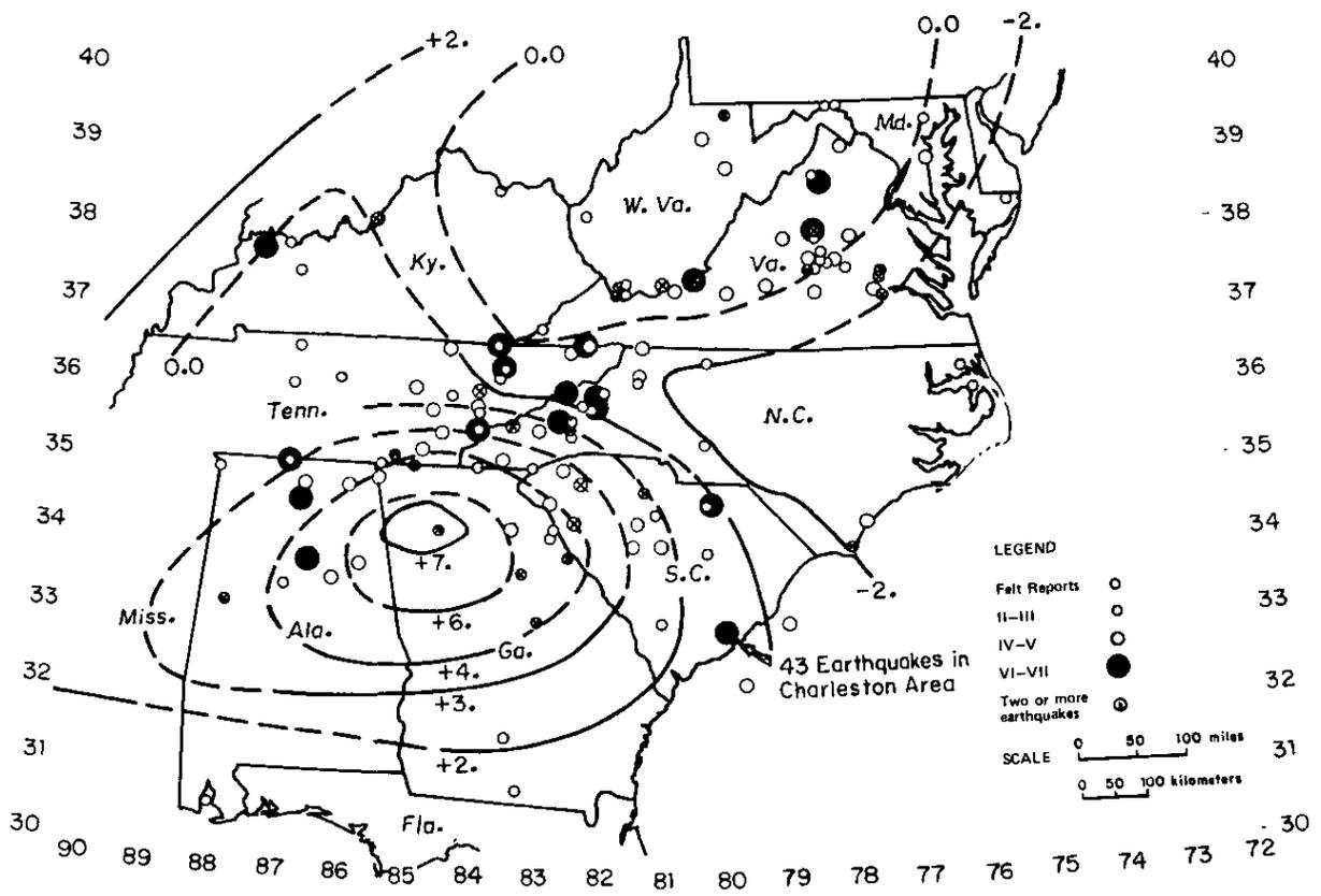
FIGURE 4. Seismicity (1920-1970) and Crustal Movement Rate for the Southeastern United States (Bollinger, 1973). Isobase Contours in mm/yr.
