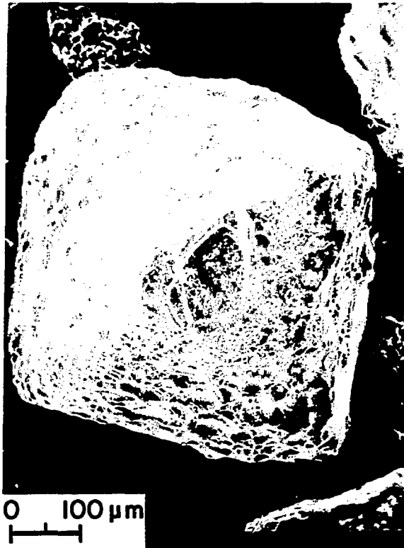
Fig. 14. Phenocryst from the Guaje Pumice Bed showing bubble wall textures. SEM photograph.
