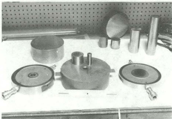
Figure 65. Piston and die assembly used for high-temperature piston-cylinder experiments. The center disk is the pressure vessel with a WC core. This core will accept a 19-mm sample assembly. The adjacent disks are the lower and upper platens containing annular segments for coolant, and connections for electrical leads.
