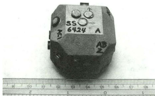
Figure 5. A Mesaverde sandstone sample with ultrasonic transducers. The three principal faces are A, B, and C. Face A is parallel to bedding. The diagonal faces AB, AC, and BC are between the corresponding two principal faces. The scale is in centimeters.
