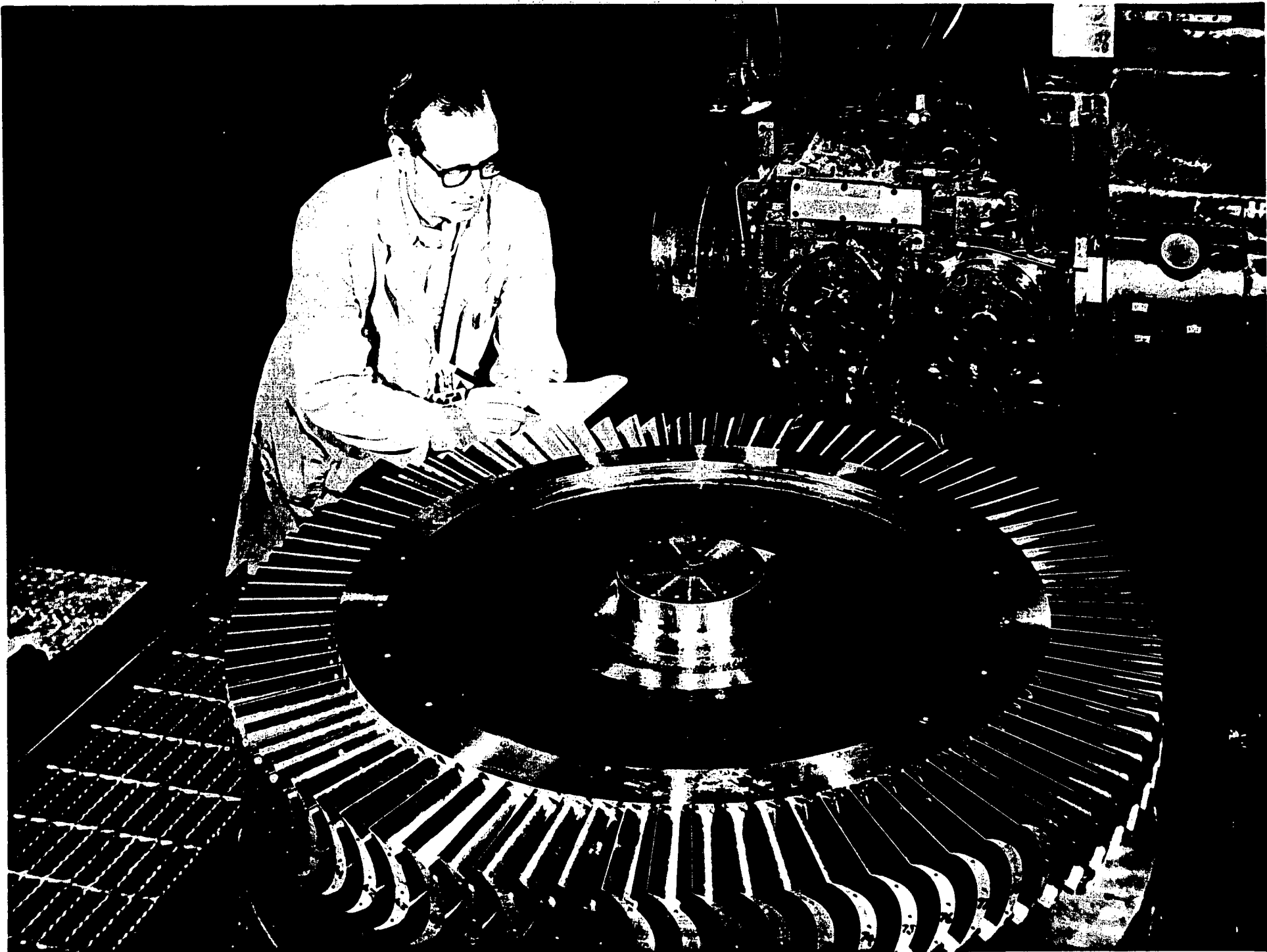
FIGURE 4-14. COMPLETED ROTOR BEFORE PLATING
