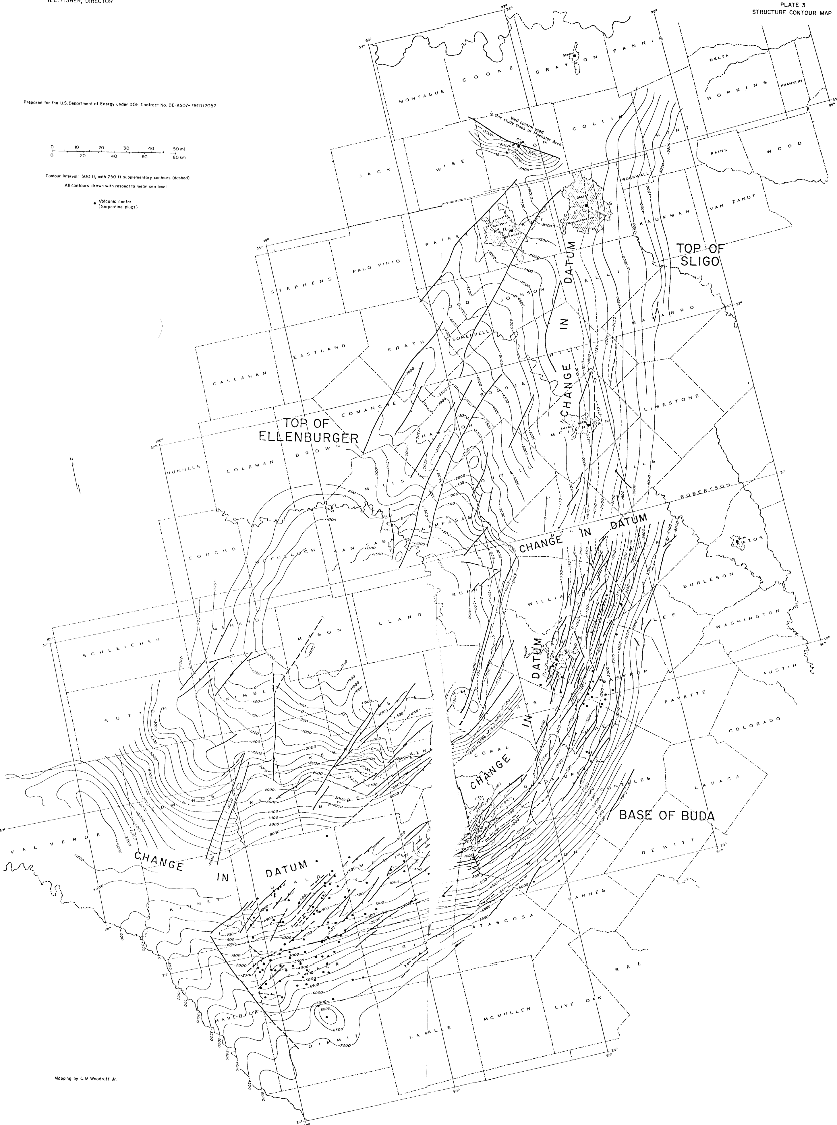
PLATE 3. STRUCTURE CONTOUR MAP OF THE BALCONES AND LULING FAULT ZONES, MEXIA AND TALCO FAULT ZONES, AND FORELAND AREAS ADJACENT TO THE OUACHITA OROGEN, TEXAS
