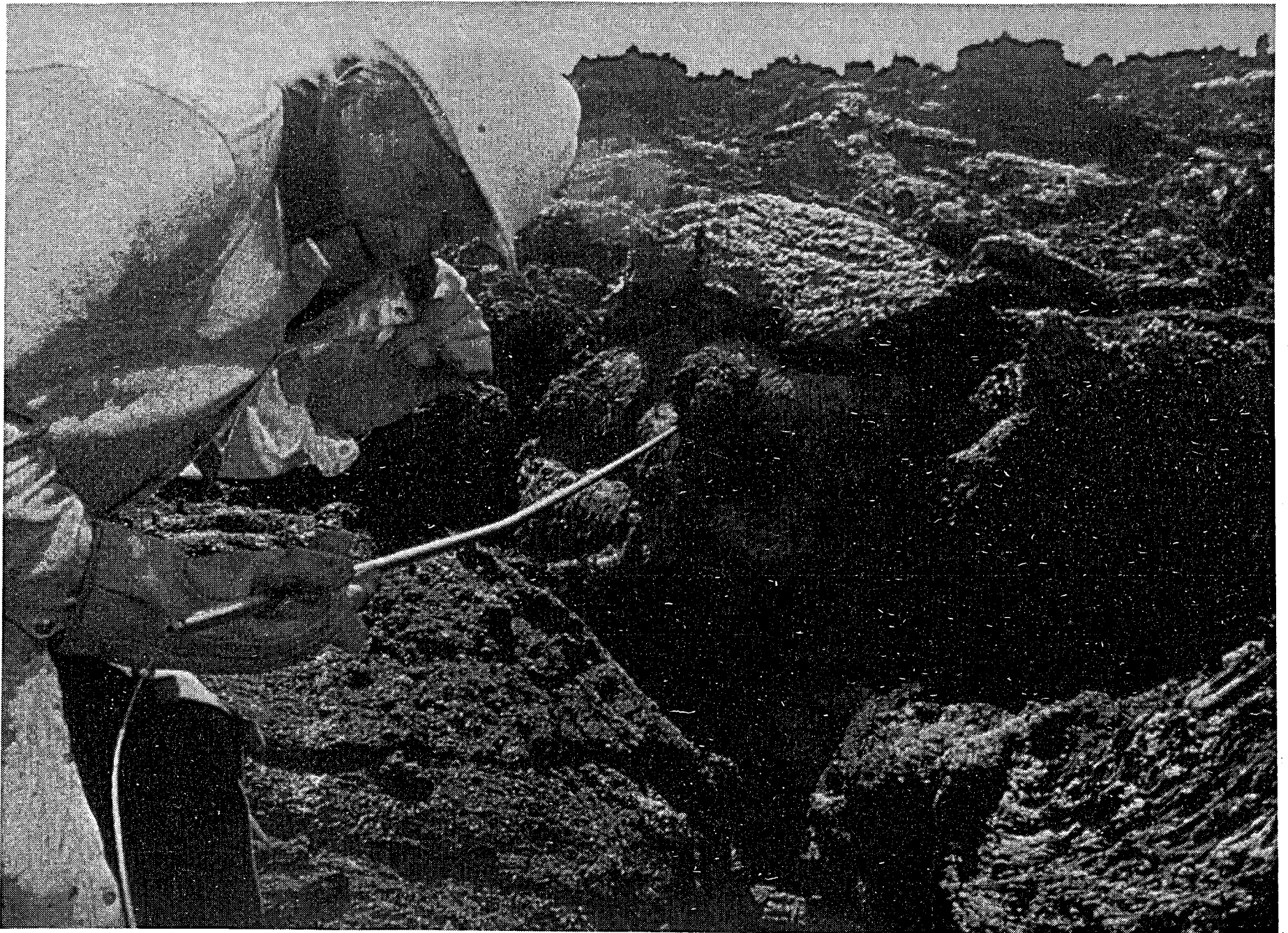
Figure 12. Transient Convection Probe in Operation in 1983 Kilauea Lava Flow.
