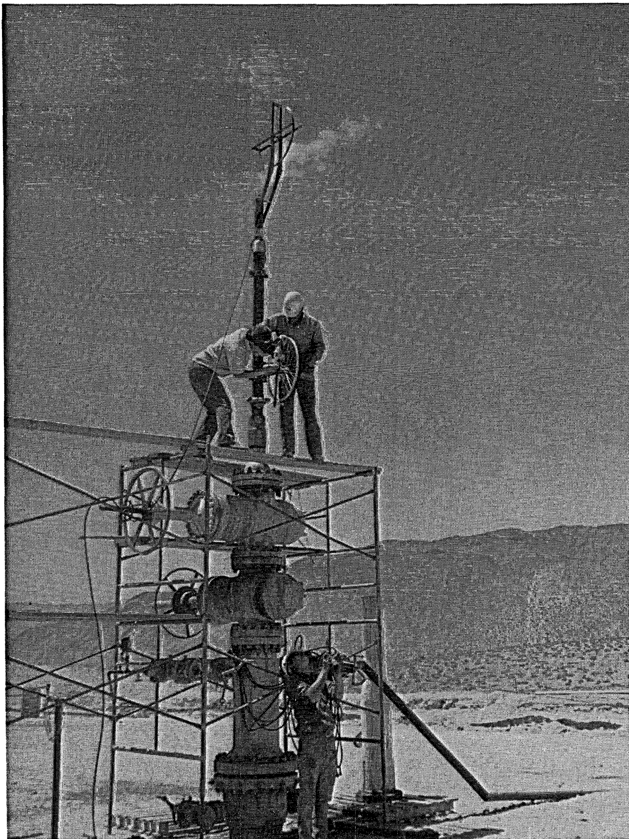
Figure 10. High Temperature Downhole Fluid Sampler Being Used to Sample in Producing Geothermal Well in Coso Geothermal Field, CA.
