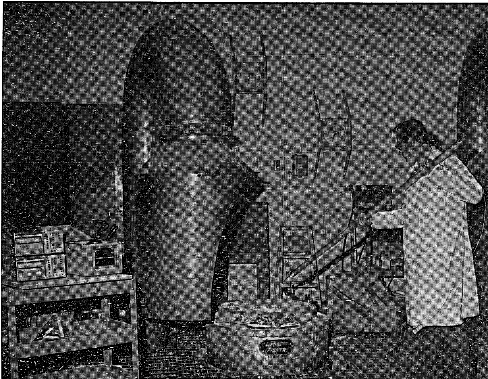
Figure 11. Laboratory Test of Transient (T2M) Convection Probe.
