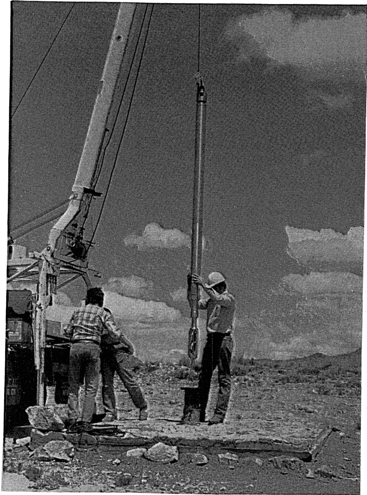
Figure 2. Downhole Seismic Source (Full Scale Model) Undergoing Tests at Buffalo Hill Test Site, Albuquerque, New Mexico.
