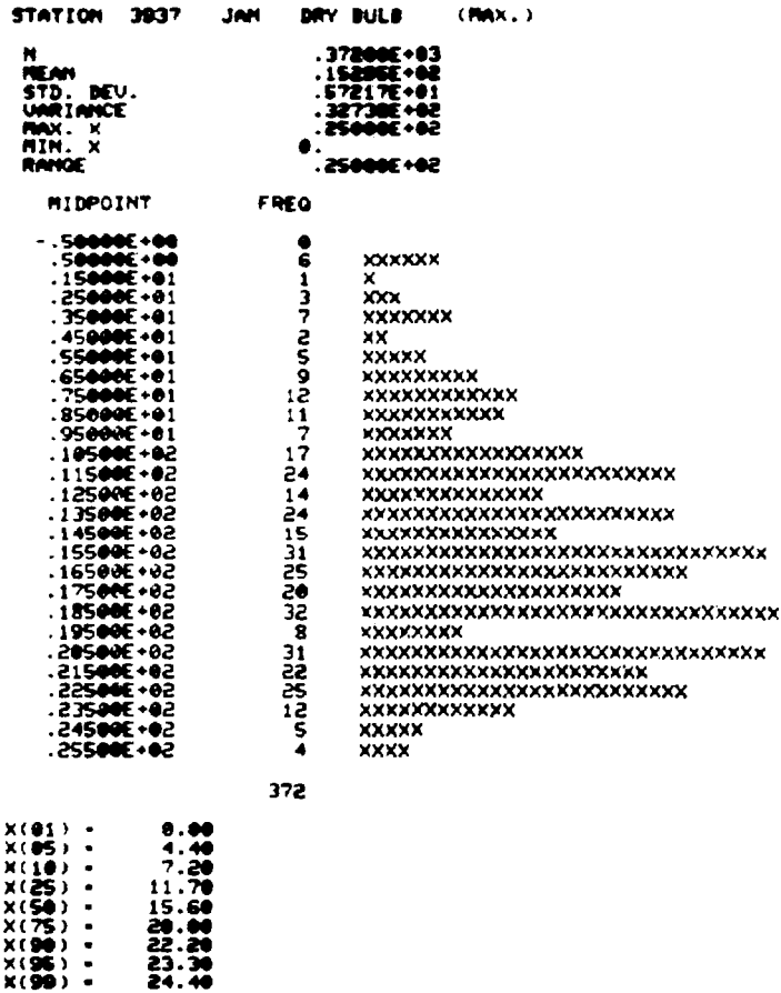
Fig. 4. Distribution statistics of January daily dry-bulb temperature maximums for Lake Charles, Louisiana, for 1953-1964.
