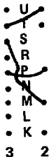
FIG. 9. Wirewrap jumpers that must be in place in PROM module location 8F.
