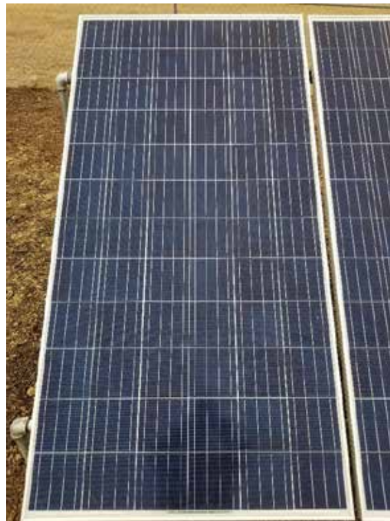
Figure 3.1 : Talesun TP672P-320 solar panel
