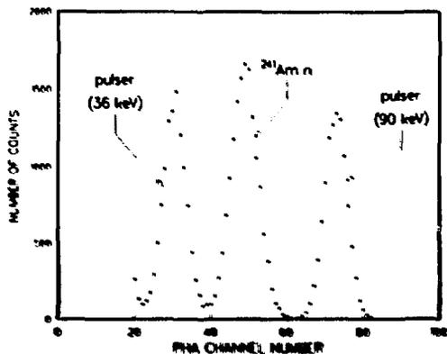
Fig. 2. PHA spectrum, showing alpha peak and two pulser calibration peaks. The data is from a 2- $\mu$ m p-i-n diode, of the type illustrated in Figure 3, biased at -90 V. The energy-equivalence of the pulser calibration peaks was determined both by direct comparison with a full-energy alpha pulse in a Si-crystal detector, and by calculation, from the measured value of the test capacitor. The two results were consistent to within 3%.
