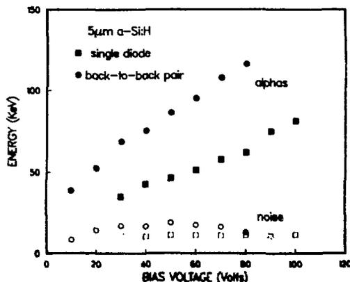
Fig. 6. Comparison of signal and noise from a single 5- $\mu\text{m}$  p-i-n detector and a stacked 5- $\mu\text{m}$  (5+5) n-i-p-p-i-p detector. Within measurement uncertainties the signal was double, and the noise unchanged, for the stacked detector.
