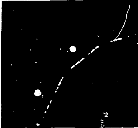
Fig. 3 - Photograph of PROTO II Switching Arc Channels
