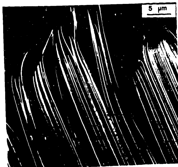
Fig. 3 Dark-field TEM photograph shows cross section of NiP alloy viewed parallel to electrodeposited layers (normal to growth direction).
