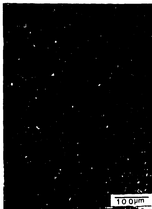
Fig. 6 Micrograph of surface of diamond-turned commercial-grade aluminum. Pits are probably result of removal of inclusions in aluminum alloy.
