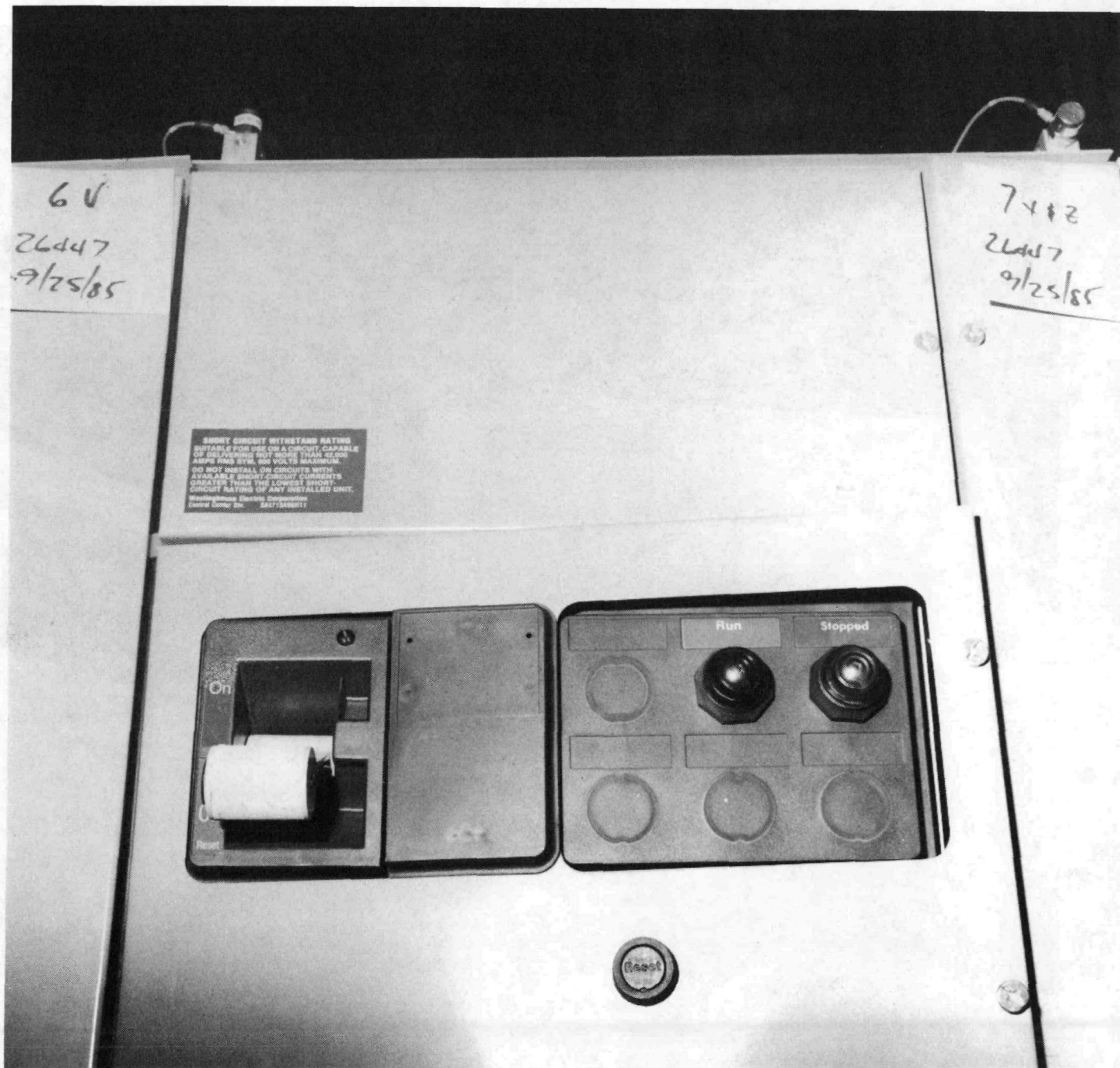
Fig. 3-4 (cont.). Accelerometer locations along top of MCC cabinet (accelerometers 6 and 7 mounted on top of cabinet).
