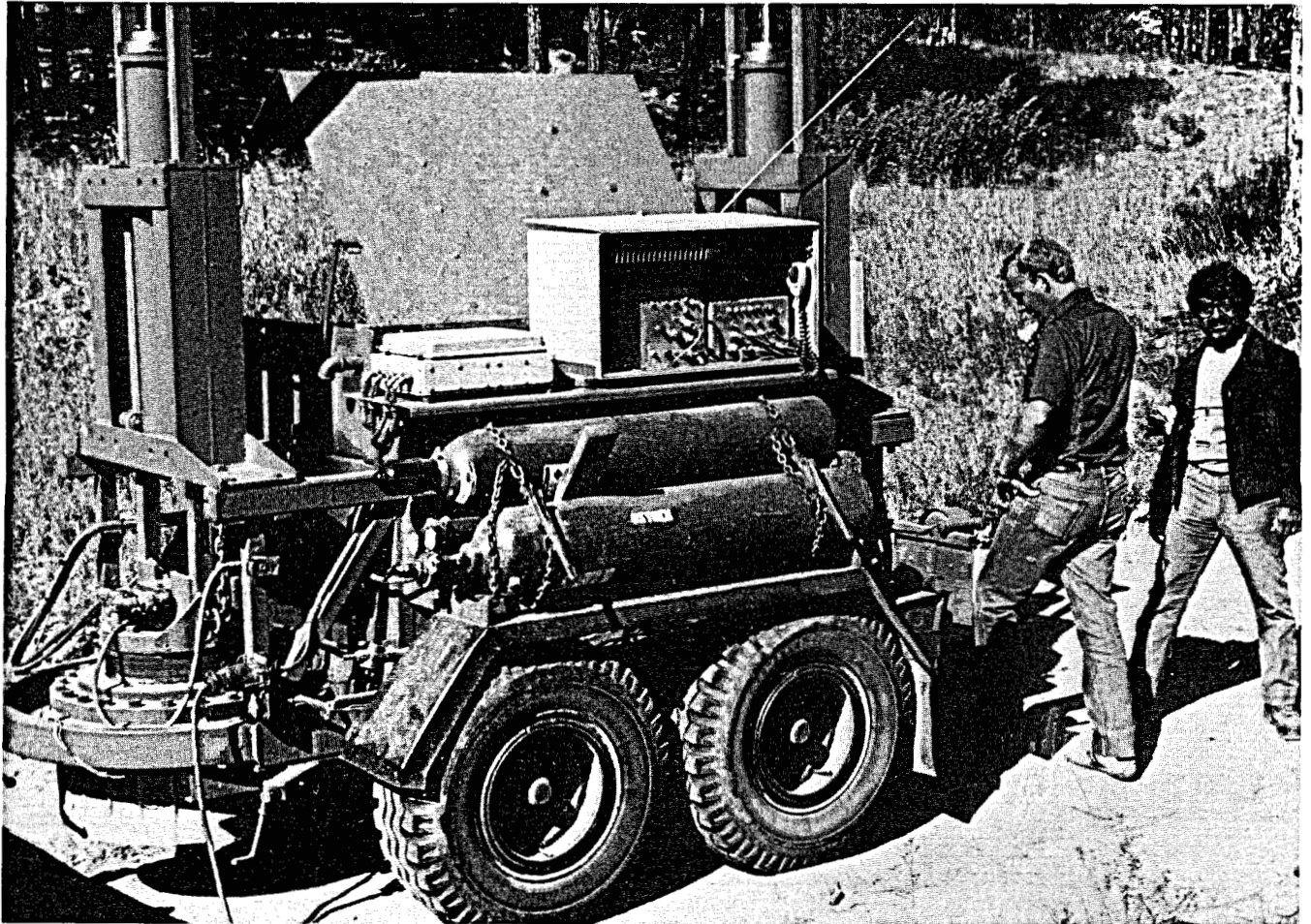
Fig. A-4. Vibroseismic equipment in operation during seismic profile, near VC-1, October 1985.
