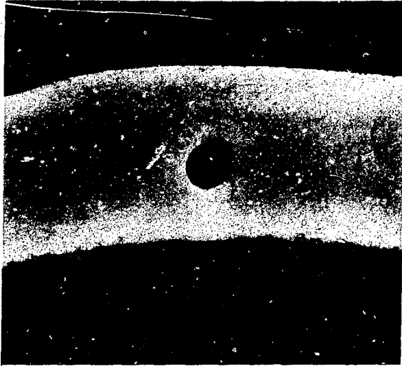
Fig. 25. A large void was observed in a transverse section removed from the SRP-423 impact face. 50X.
