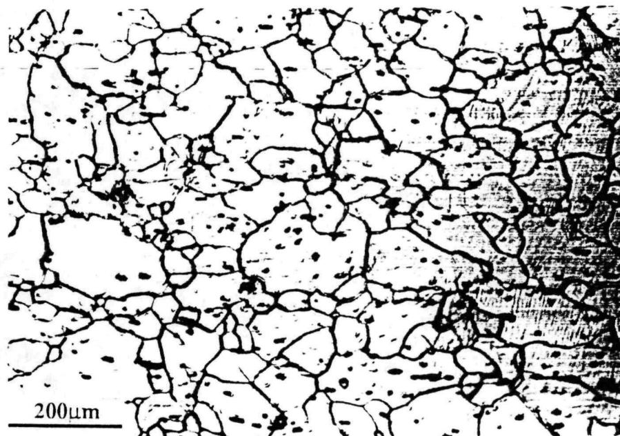
Fig. 3.36. The optical microstructure of the side surface of the specimen tested at 2400 K.
