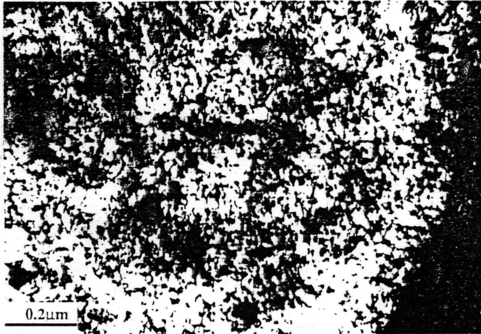
Fig. 3.17. Numerous fine precipitates were formed in the 1955 K creep tested sample.
