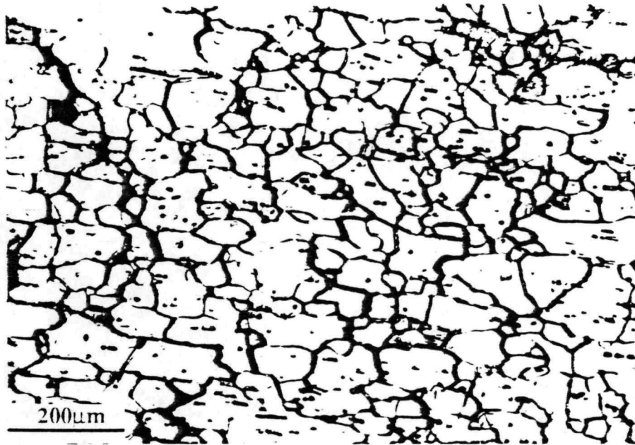
Fig. 3.35. The optical microstructure of the side surface of the specimen tested at 2300 K.
