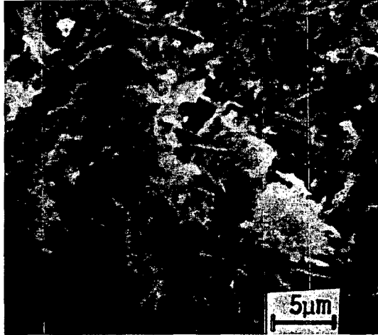
Figure 5. Interlocking needles of xonotlite formed from \beta - C_2S + tripoli at 48% CaO, 52% SiO 2 cured at 350°C, 68.9 MPa for 10 days.
