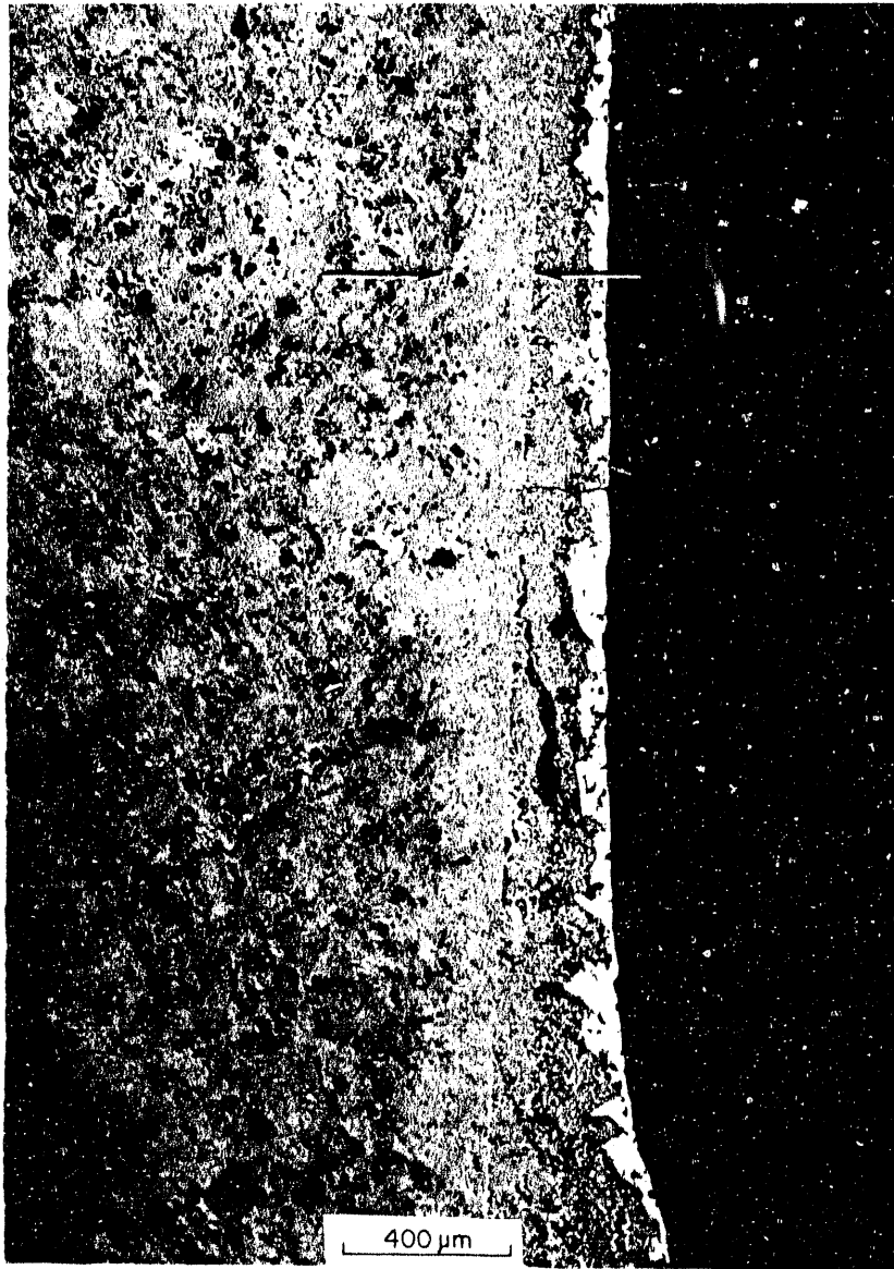
Fig. 9. Mg 2 Si-Si eutectic alloy forming a thin meniscus on the inner surface of a Stackpole 2020 test capsule. Note restructured layer in the graphite (arrows).
