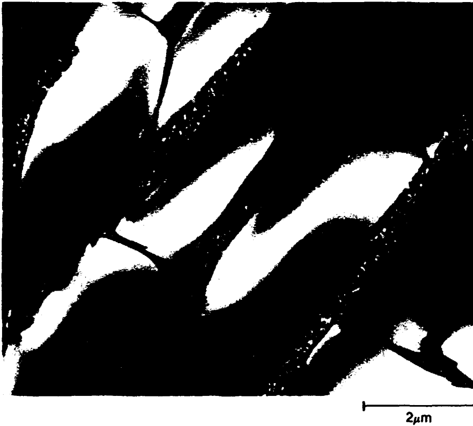
Figure 4. Superlattice dark field of disordered webs in \text{Ni}_3\text{Al} + \text{Cr} after annealing at 1200^\circ\text{C} for 1 h.
