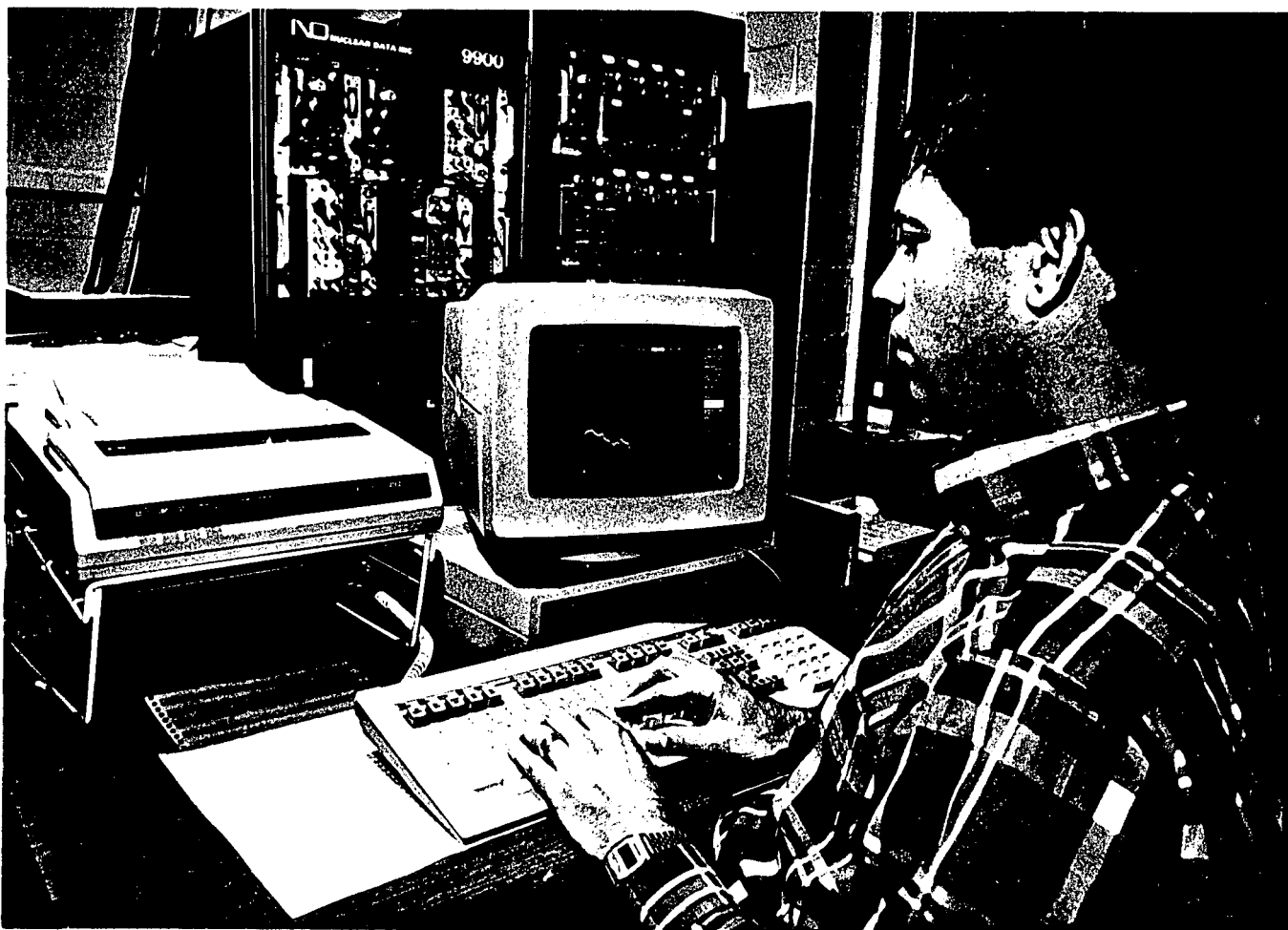
Figure 4. A microcomputer-based spectrometer system, vintage 1980.
