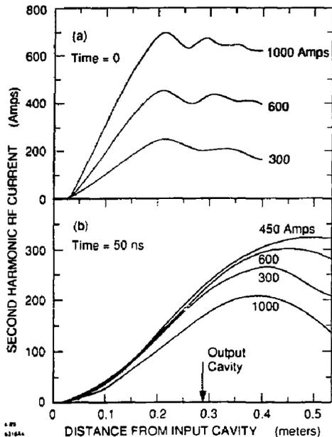
FIG. 1. Calculated second harmonic (11.4-GHz) RF current downstream from the SHARK input cavity for several different DC beam currents (a) immediately after turn-on of a DC beam of 1-MeV kinetic energy, and (b) after 50 nsec of uniform DC beam current.
