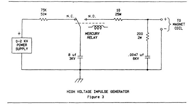
storage oscilloscope and photographed or plotted. Any change in the waveform will indicate a turn-to-turn breakdown of insulation. This test is usually done before and after the collaring operation, and should not be repeated any more than necessary to avoid stressing the insulation. As mentioned before, a resistance test of the main coils is made before and after this test.
