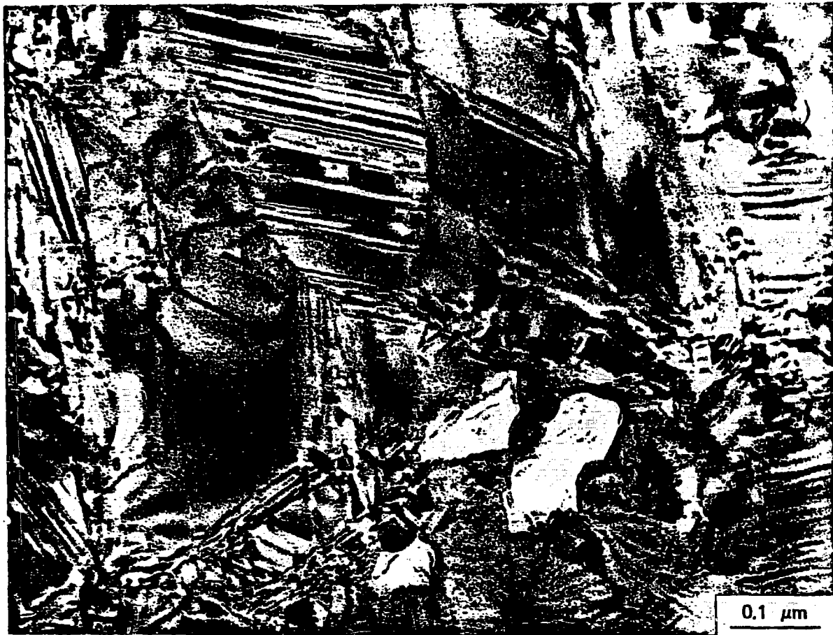
Fig. 1. Pyrolytic \beta -SiC, as deposited. Growth direction is upward. Note stacking faults and small cavities.
