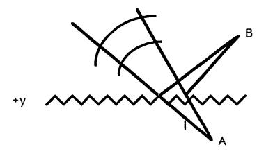
Fig. 2. Geometry of wavefronts onto VLS grating.
