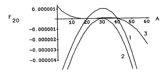
Fig. 3. The defocus aberration as a function of wavelength for the three different focal conditions.
