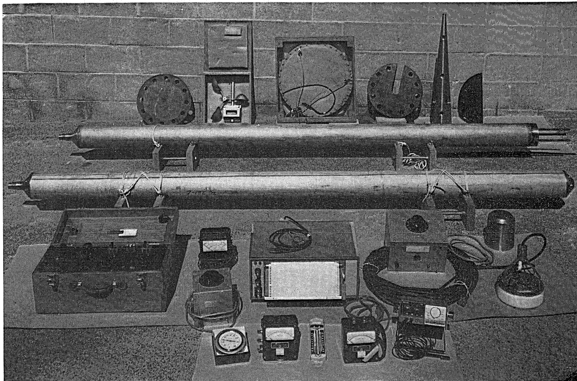
Figure 10. View of the two downhole transducers along with associated support equipment.
