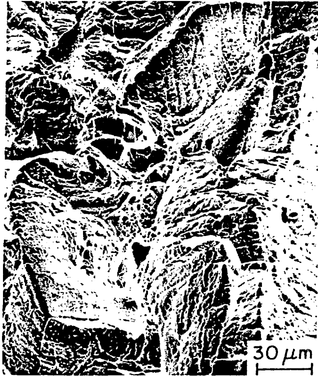
Figure 7 - Fracture Surface of Impact Test Specimen of Reannealed KRB Material Tested at Room Temperature.
