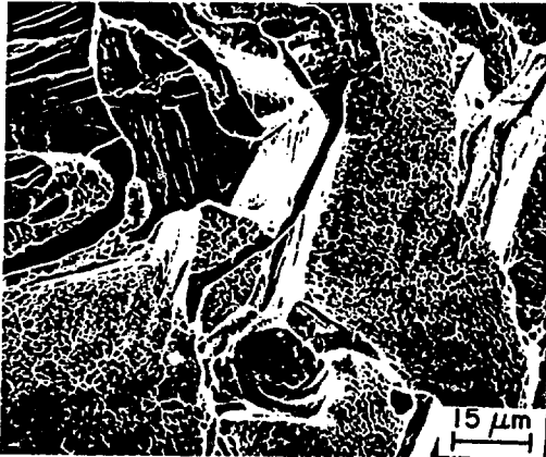
Figure 3 - Fracture Surfaces of Impact Test Specimens of Unaged CF-8 Cast Steel Tested at -196^{\circ}\text{C} .
