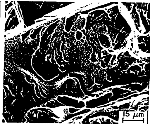
Figure 3 - Fracture Surfaces of Impact Test Specimens of Unaged CF-8 Cast Steel Tested at -196^{\circ}\text{C} .
