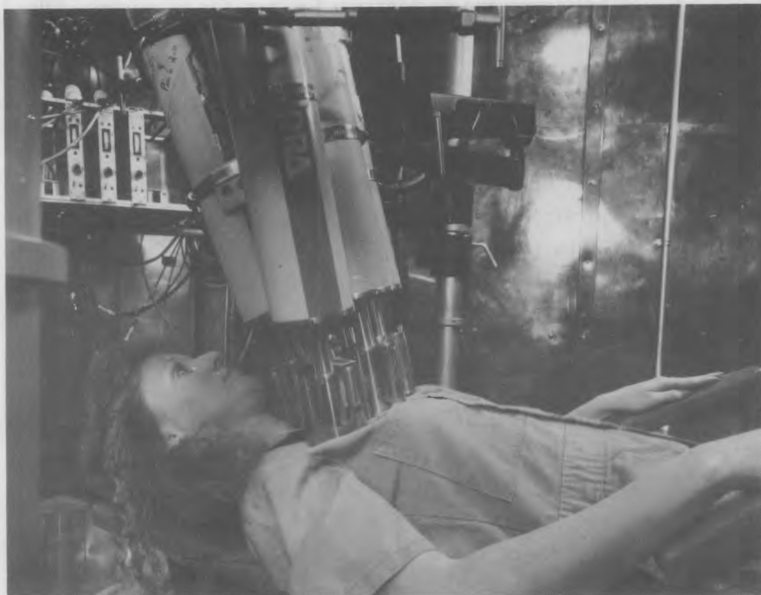
FIGURE 11. Supported Planar Germanium Detectors in Use on a Subject
