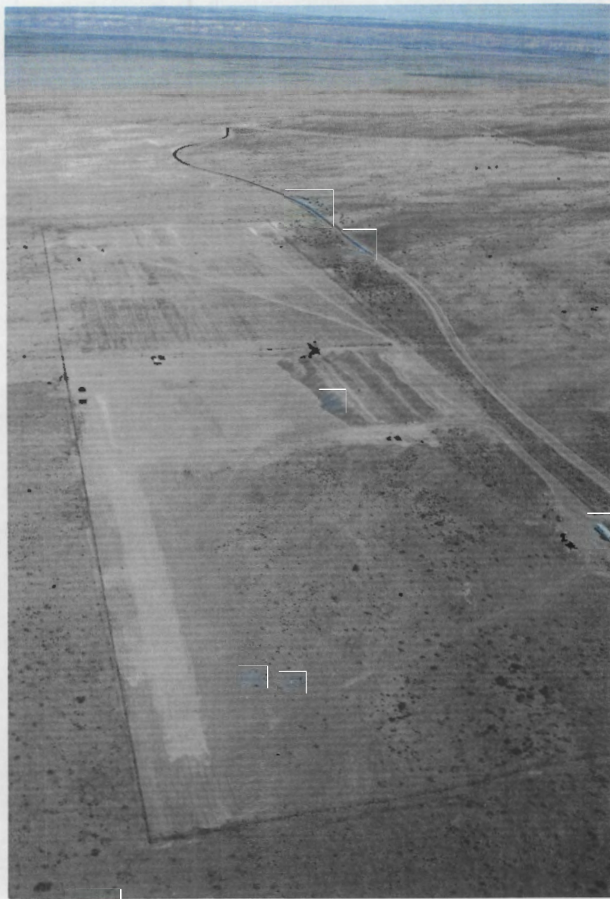
FIGURE 3. Aerial View of Hanford's Solid Waste Landfill and Nonradioactive Dangerous Waste Landfill, Looking Northeast Across the Pasco Basin. The rectangular outline includes the Solid Waste Landfill (center and foreground); and the Nonradioactive Dangerous Waste Landfill, along the northern edge. Note the active trench in the Solid Waste Landfill in the center of the photograph. The section with the diagonal road across it is the closed Phase I section of the Solid Waste Landfill.
