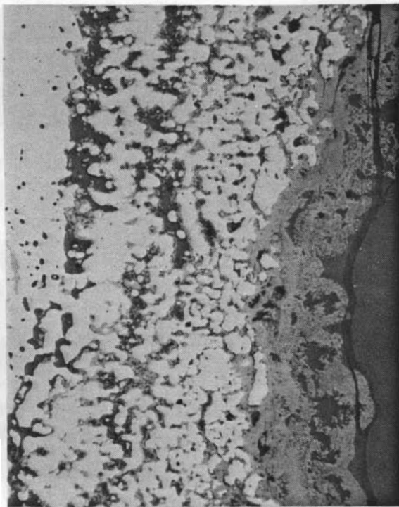
FIGURE A.108. Inconel-601 Cross Section Under 100X and 250X SEM Magnification
