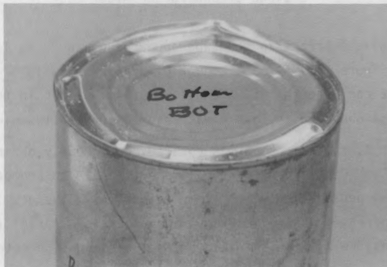
FIGURE 15. Distortion of No. 2-1/2 Can Due to Pressure During Heat Test
