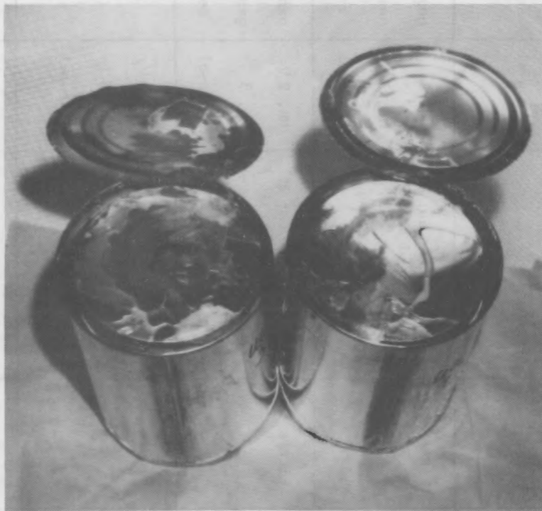
FIGURE 12. Remnants of Polyethylene Bags that Melted During the Heat Test
