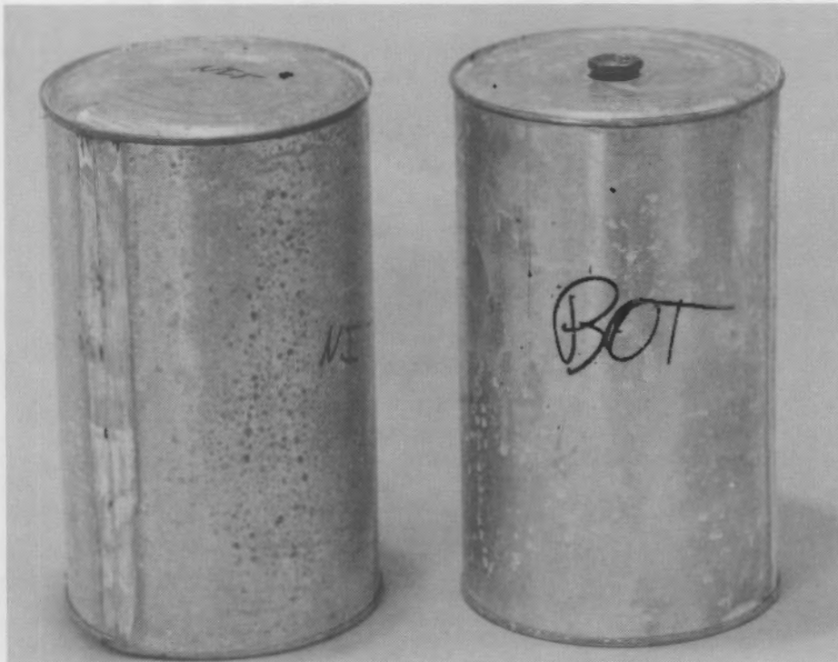
FIGURE 14. Number 3 Cans After Impact and Heat Tests (test 5, left; test 4, right)
