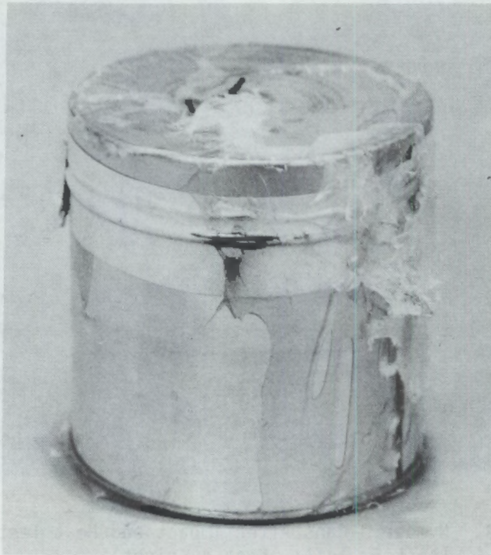
FIGURE 16. Condition of Tape Seal Showing Leakage of DUO Powder After Leak Test
