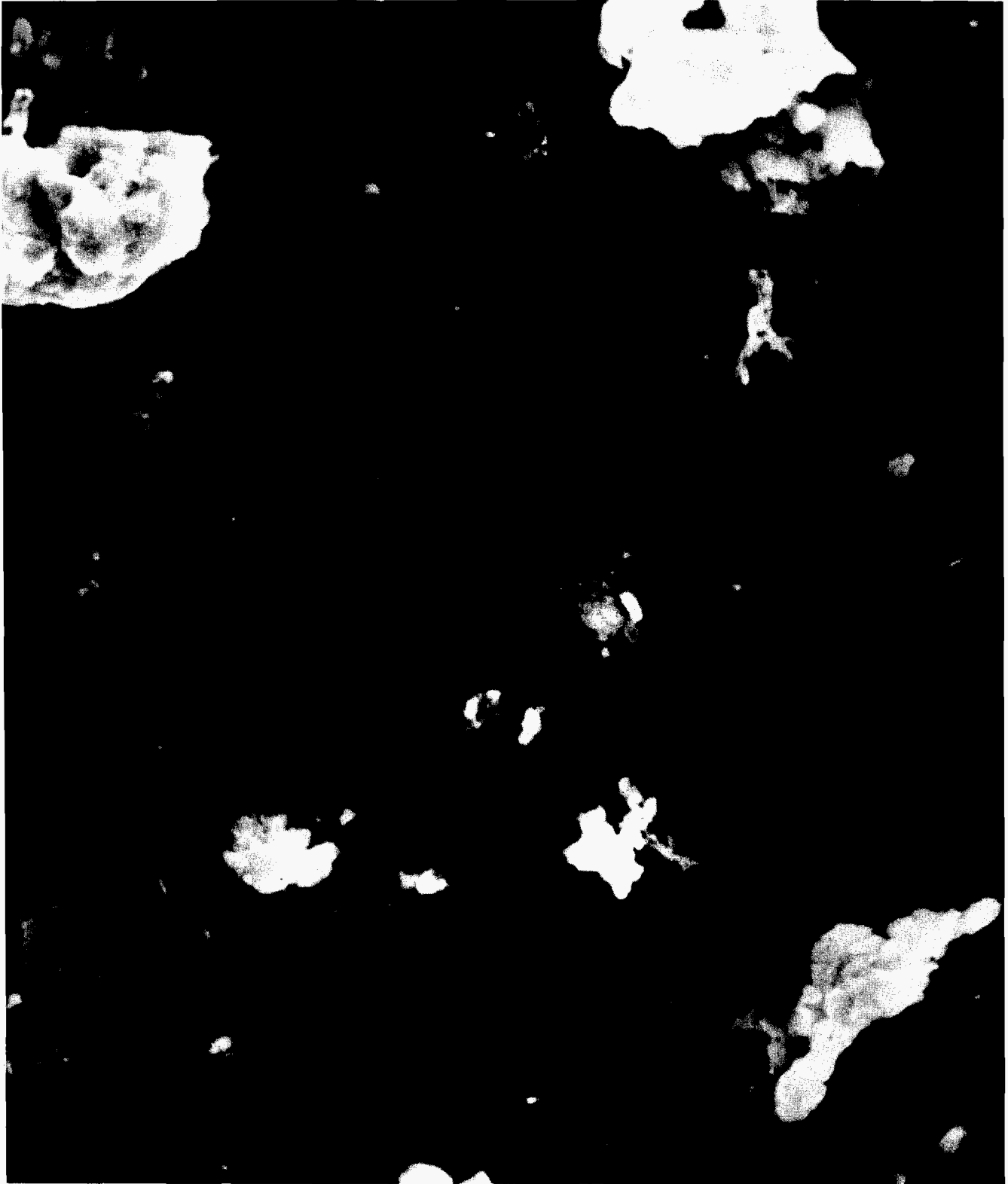
FIGURE 2.17. SEM 1500X. Composite Sample (#6, #7, and #18) - Fraction <10\ \mu\text{m} LLD - Field #1, Typical Size and Shape of Particles
