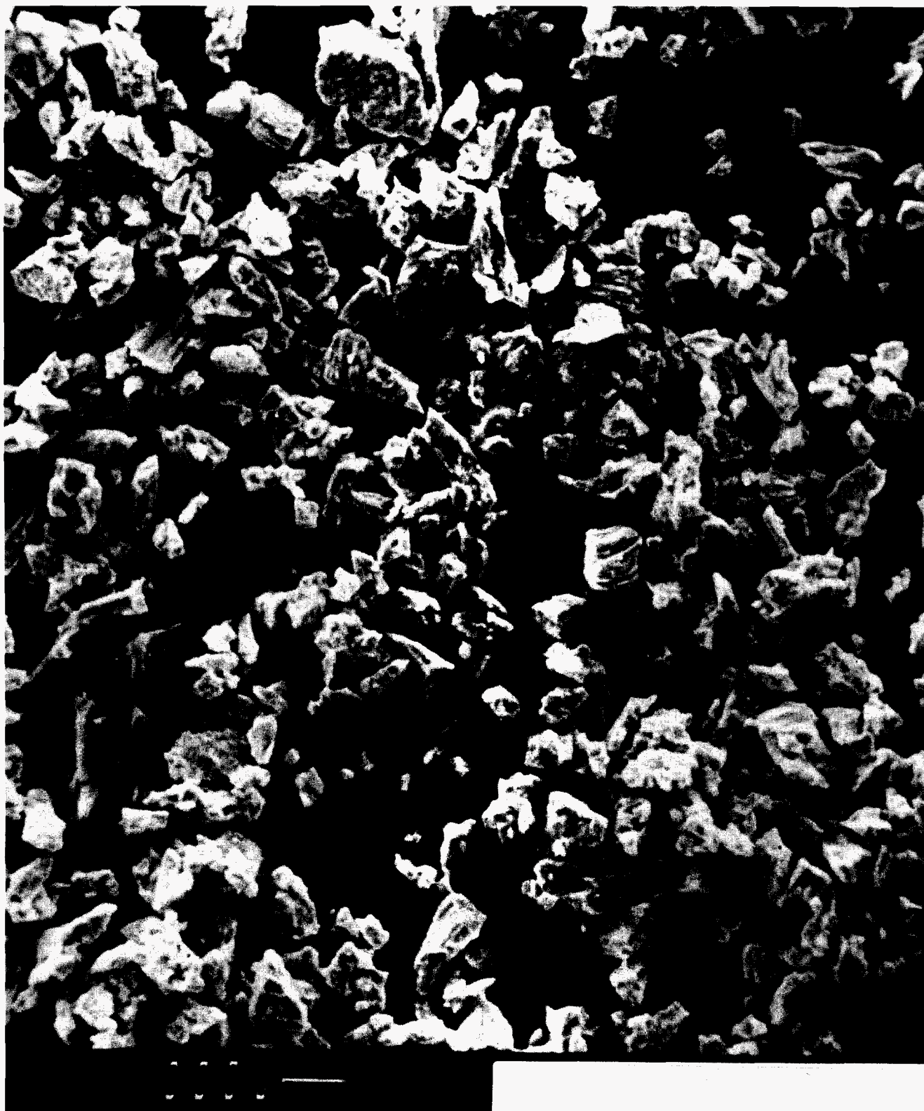
FIGURE 2.15. SEM 500X. Particle Size Analysis Sample - Fraction < 10 \mu\text{m} LLD - Field #1, Typical Size and Shape of Particles
