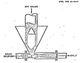
Fig. 5. Revised mixer solids feed.
