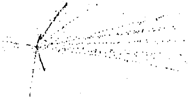
Figure 3. A Typical particle interaction image is shown. Note the low percentage of pixels which are of interest. This type of image lends itself to image compression with good results.
