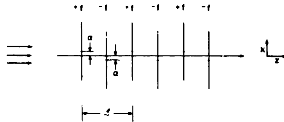
Fig. 1. Periodic thin-lens array used for simulation.
