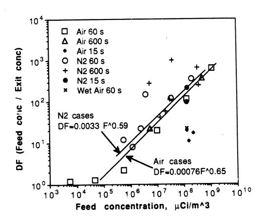
Fig. 5 Data of Tritium Decontamination Factor
