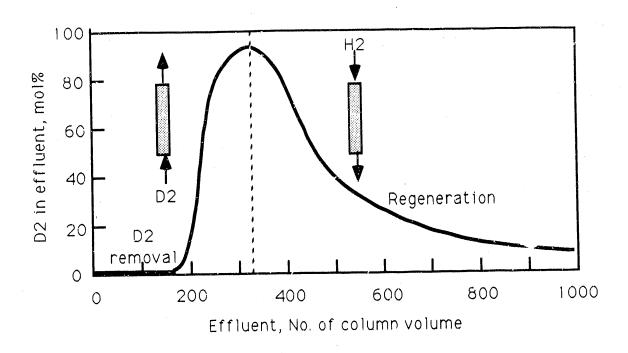
Fig. 4 Breakthrough Curve and Regeneration of the Catalytic Exchange Stripper
