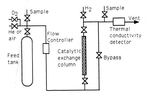
Fig. 2 Schematic of the Catalytic Exchange Stripper for D<sub>2</sub> (Cold) Tests
