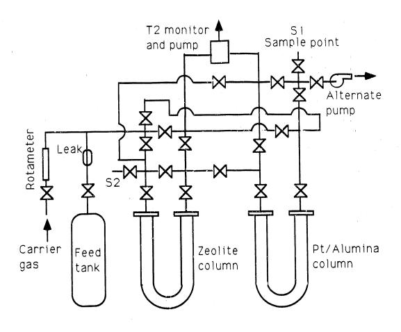
Fig. 3 Schematic of the Catalytic Exchange Stripper for T<sub>2</sub> Tests
