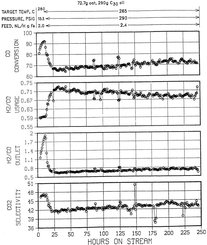
PLT 700B RUN 31 H<sub>2</sub>:CO feed = 0.7, 1100 rpm
