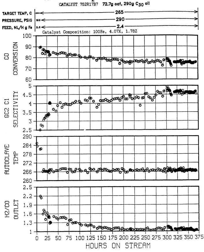
PLT 700B RUN 33  $H_2$ :CO feed = 0.7, 1100 rpm
