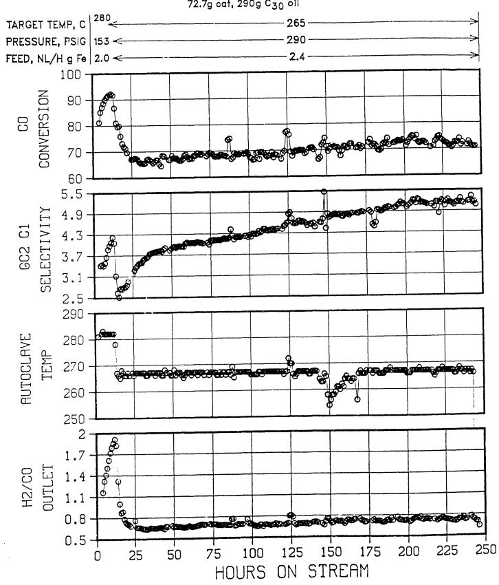
PLT 700B RUN 31  $H_2$ :CO feed = 0.7, 1100 rpm 72.7g oat, 290g  $C_{30}$  oil
