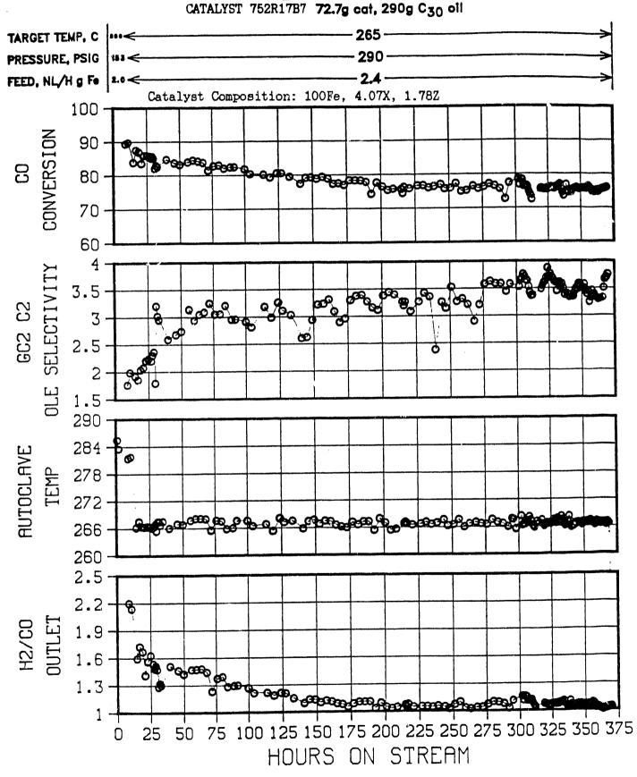
PLT 700B RUN 31 H<sub>2</sub>:CO feed = 0.7, 1100 rpm
