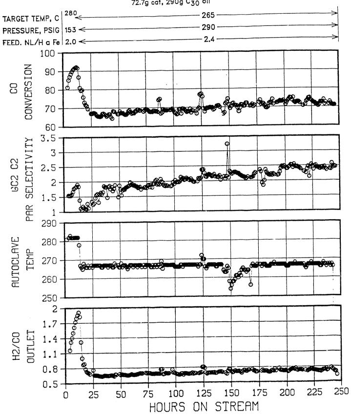
PLT 700B RUN 31  $H_2$ :C0 feed = 0.7, 1100 rpm 72.7g cat, 290g  $C_{30}$  oil
