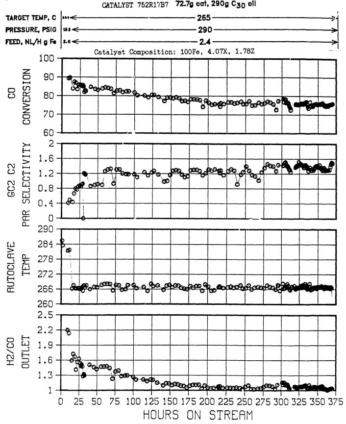
PLT 700B RUN 33 H<sub>2</sub>:CO feed = 0.7, 1100 rpm
