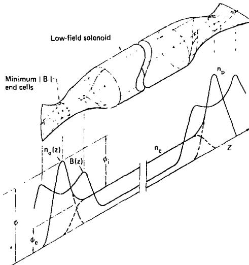
Fig. 2. Tandem mirrors with umbipolar barriers at the ends.
