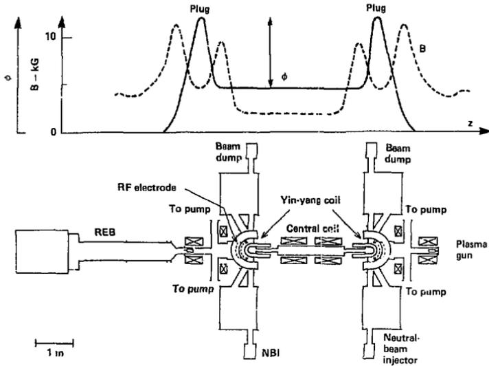
Fig. 3. Schematic diagram of Gamma 6 experiment (Miyoshi and co-workers, 1978).
