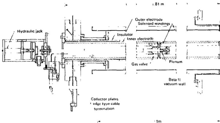
Fig. 9. Diagram of Beta II plasma gun.
